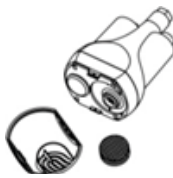
Clean the filter net (5) and filter cover (6).
